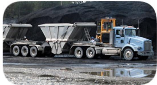
*Coal trucks, similar to the ones that currently travel the Island Highway every day, could be used to transport the coal from the Raven Project. They would be covered to eliminate coal dust and would connect directly to the Inland Island Highway using industrial roads.*
